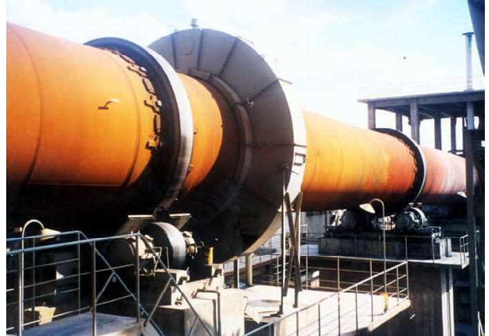
Open gearing, such as this huge ring gear that drives this rotary cement kiln, pose special lubrication challenges ... SWEPCO 164 solves them.
